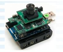
Citric Platform (Berkeley) Sensor: 1280 x 1024 @ 15 fps (640 x 480 @ 30 fps) CPU: Intel XScale PXA270, max 624 MHz, 32-bit FLASH: 16 MB, RAM: 64 MB
